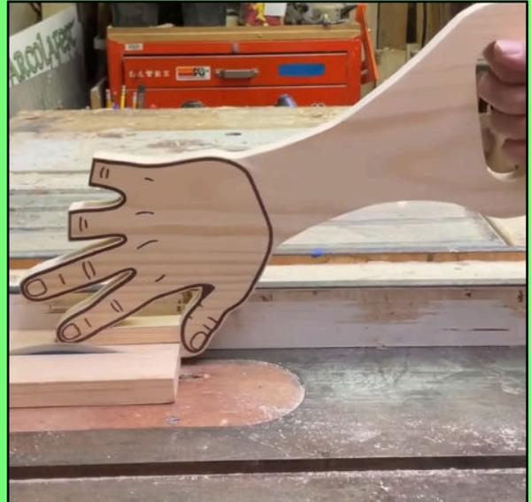
A handy device for pushing timber through a saw. Note missing fingers!
